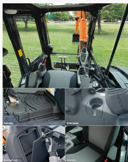
Shown equipped with cab, suspension seat, armrests, FM/AM radio, auxiliary function lever, air condition and pedal as optional items.
